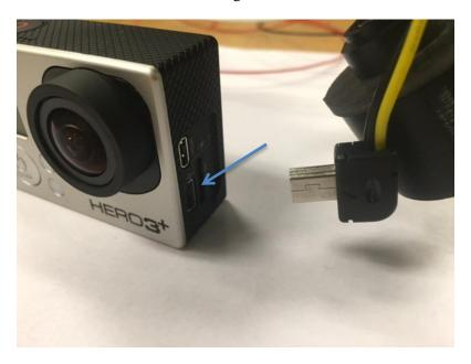
C) Once plugged in, slide the camera into the gimbal, in the direction indicated by the arrow. The camera should slide on easily, and does not require much force. Ensure that the camera has the correct orientation, as shown in the image below.
