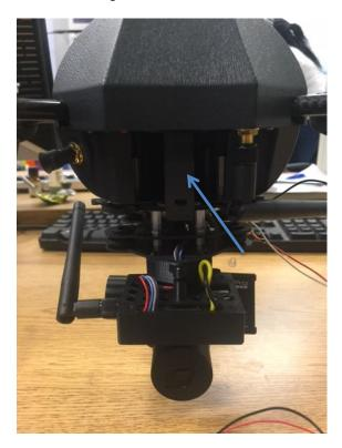
C) Slide the battery into the slot, making sure the red and black connecting wires are on the left, as shown below. The battery should slide in easily and should not require much force.
